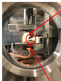
Side-view into the vacuum chamber of the AFM.
