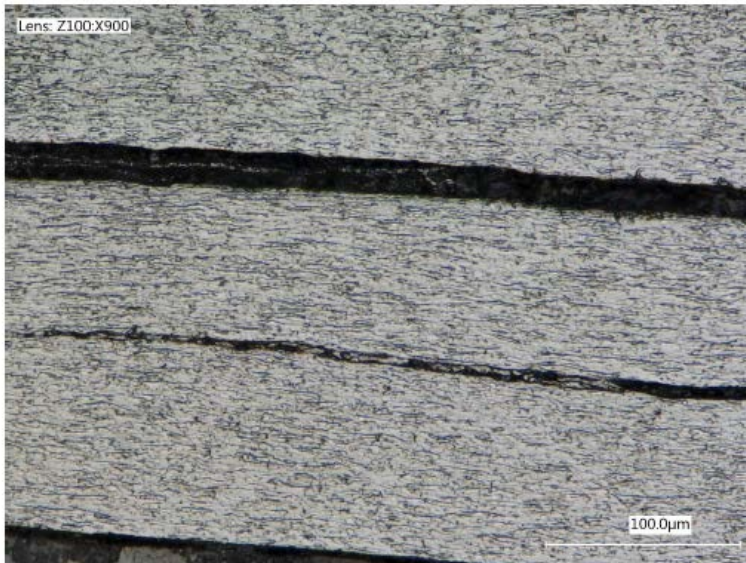
Microstructure in the defect zone.
