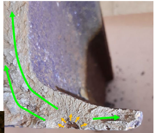
Pitting corrosion, Hemtunnel, J.vd Stelt, 2020
