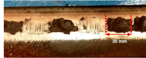
Typical spalling in MHH steel after grinding, (Dekra Rail, 2016)
