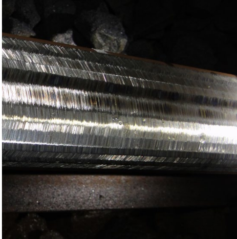
Freshly ground rail surface of a British Steel R370CrHT rail. Surface roughness and ground facets are clearly visible [Schotsman2017].
