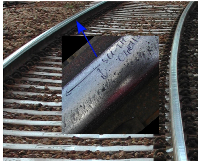
Gauge corner cracking, S. Grassie
