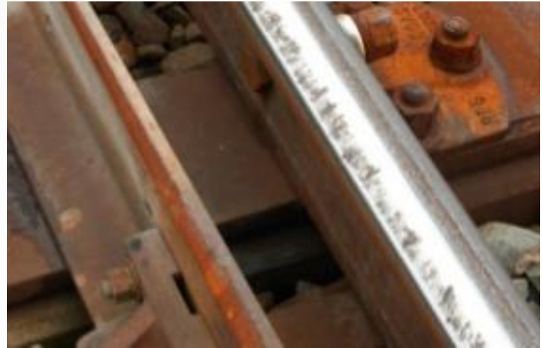
RCF damaged stock rail
